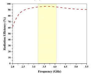
Figure 4: Simulated Efficiency Vs Frequency of Proposed Antenna
