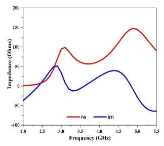
Figure 6: Impedance characteristics of the proposed antenna
