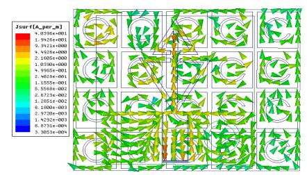
Figure 3: (a) Antenna Current Distribution (b) Antenna Current Magnitudes
