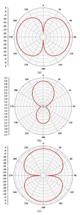
Figure 8: Simulated Radiation Pattern (a) XY-Plane (b) YZ-Plane (c) ZX-Plane
